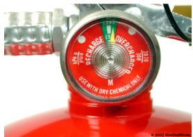
❖ Extinguishers have a life span of 10 to 12 years. The date of manufacture will be on the extinguisher, either on the bottom or on the label. Have it serviced or replace it with a new one.
