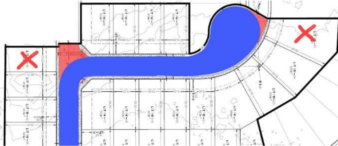
Figure 11-1 - Snow Clearing Path and Driveway Access
